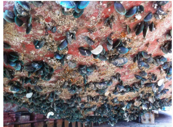
Figure 2 Underside of a vessel hull, fouled with mussels, source Biofouling Solutions (A. Coutts)
